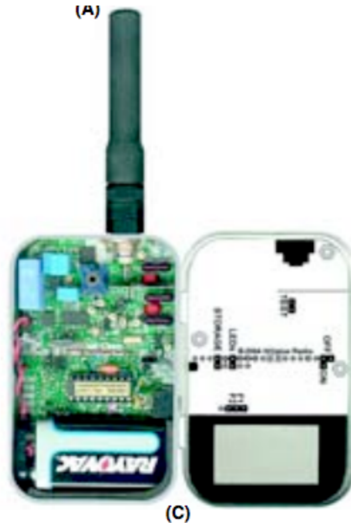
Fig 2—Views of the project. A is an outside view of the Pocket APRS Transmitter with antenna and GPS receiver. B shows a side view with the GPS port jack. C is an internal view of the Pocket APRS Transmitter.
